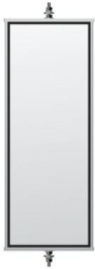
Item No. 60007 6" X 16" 430 Stainless Steel West Coast Mirror - Non Heated MSRP: $ 21.99 OEM No. :
